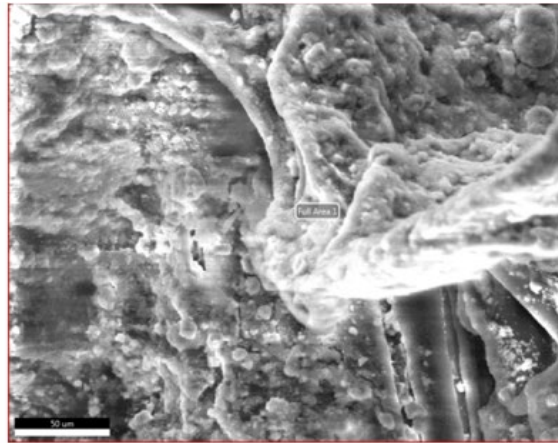
Figure 7.3. 10%HAp (w/v) and conjugate 5% gelatin- KRSRGYC (w/v) coated suture's EDS result obtained from SEM.
